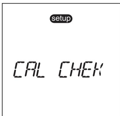
Allows the user to confirm the last calibration for the selected measurement mode.
