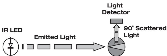
**Figure 1. Pure Nephelometric Turbidity Measurement without Color Compensation**
