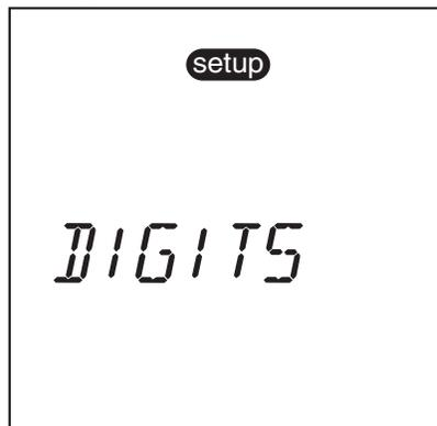
The digit selection allows the user to select the resolution of the reading, from 0.000, 0.00, 0.0 and 0 or auto resolution. Default is auto resolution.
