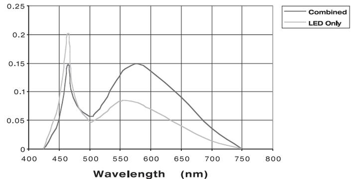
As can be seen from the graph, the white LED – Si photo detector system described here is quite broadband. Its appearance is very similar to that of a tungsten bulb and a cadmium sulfide photo detector combination. It also contains a narrow secondary peak at 460 nm. As the blue output is very limited in tungsten bulbs, this peak can aid in better detection of very small particles. However, as the peak area is very small compared to that of a main body, this enhancement is not very pronounced.
