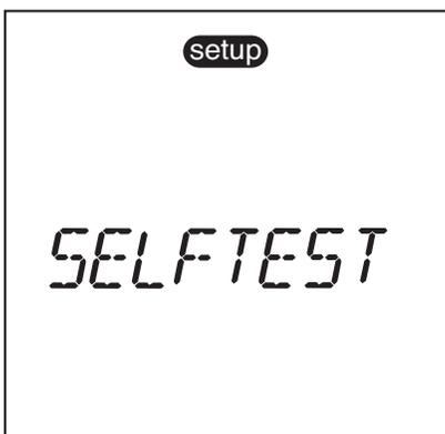
Puts the turbidimeter into a self-diagnostic mode. See the **Turbidimeter Self Test** section.
