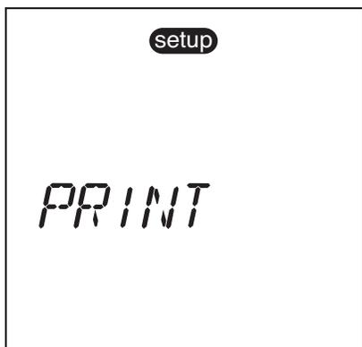
Allows the user to select the printout format. The user can select between a standard printout or a comma delimited format for importing data into a spreadsheet.
