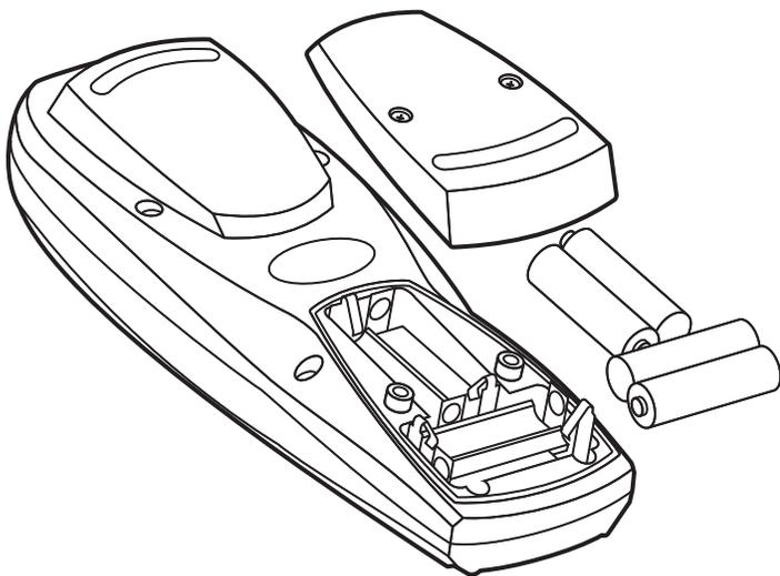
**Figure 5. Battery Installation**
