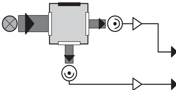
**Figure 2. Color Compensation in the Dual-beam System with Two Photo Detectors**
