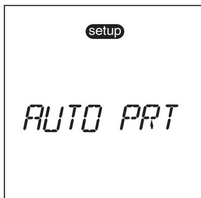
Auto print “ON” will automatically send readings to the printer.
