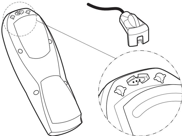
**Figure 9. AQ450 RS232 Cable Connection**
