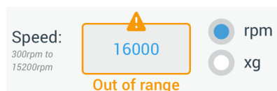
Figure 3-16: Settings -&gt; Controls -&gt; Setpoints Screen: Out of Range Value Alert
