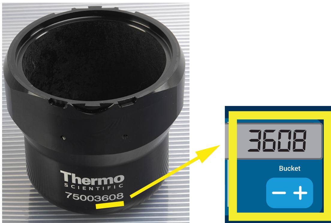
Figure 2-18: Setting the Correct Bucket Code
