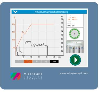
easyTEMP temperature control of an exothermic reaction during the digestion of an API with HNO<sub>3</sub> and HCI in the SK-15 rotor
