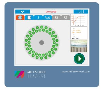
This rotor diagram represents the digestion temperature in all vessels. The green color indicates if the vessel has achieved the set conditions
