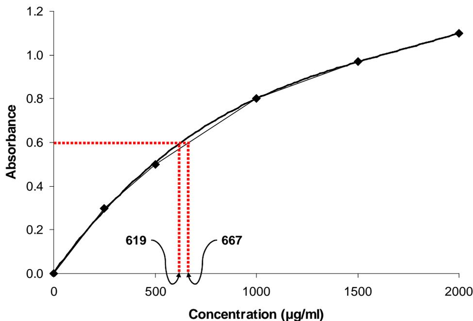
**Figure 2.** Example standard curve involving six points. The thin line is a point-to-point graph through the plotted standards. The thick line is a 3-parameter regression for the entire set of standard points. Dashed lines represent interpolations for a test sample having absorbance 0.6. See text for additional details.
