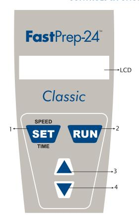
1. SET Key - Press this key to select Speed & Time as displayed on LCD and to choose program (model 6004)
