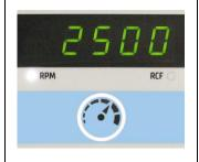
• Rotational speed (indicator RPM is lit)
