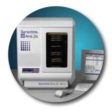
Thermo Scientific Sensititre ARIS 2X System. The ARIS™ 2X System is a fully automated, benchtop incubating and reading system that reduces workload and facilitates efficient workflow. It can accomodate 64 MIC, breakpoint or identification plates, for a combination of 192 possible tests on a single instrument.
