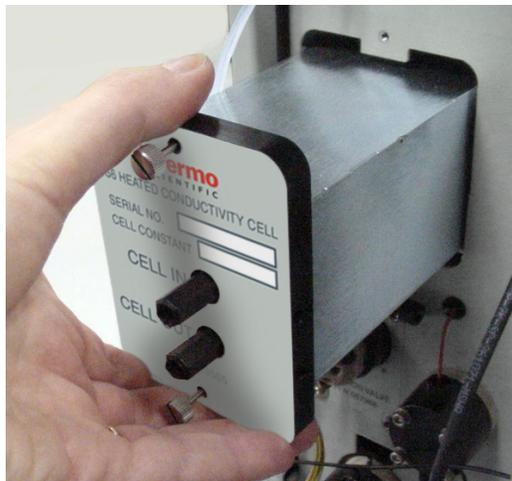
6. Slide the new cell assembly straight into the opening in the component panel until it stops and the cell cover is flush against the component panel.
