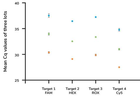
**Figure 6.** Results from lot-to-lot consistency tests with 4-plex RT-qPCR reactions over three 10-fold RNA dilutions (0.1 ng/rxn, orange; 0.01 ng/rxn, green; 0.001 ng/rxn, blue). Mean Cq values across three different production lots along with standard deviations are presented (if SD>0.16).
