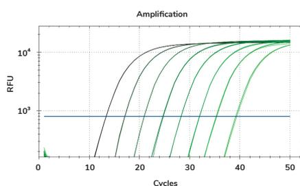
**Figure 1.** PPIA target from human total RNA was amplified over eight 10-fold dilutions (1000 ng to 100 fg,  $R^2=1.0$ ), showing sensitive detection over a wide dynamic range. Reactions were ran on Bio-Rad CFX96 platform.
