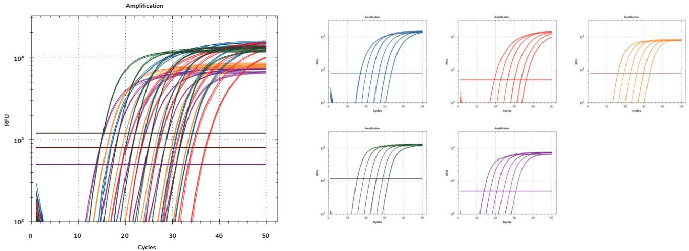
**Figure 3.** Five-plex RT-qPCR reactions (FAM, blue; HEX, green; ROX, red; Cy5, purple; Cy5.5, orange) on Bio-Rad CFX96 platform with six 10-fold serial dilutions of reference human total RNA (from 1000 ng/μl to 0.01 ng/μl).
