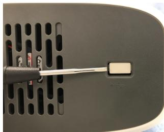
Figure 3 USB port dust cover (Rear view of PowerEase™ Touch 120W Power Supply)
