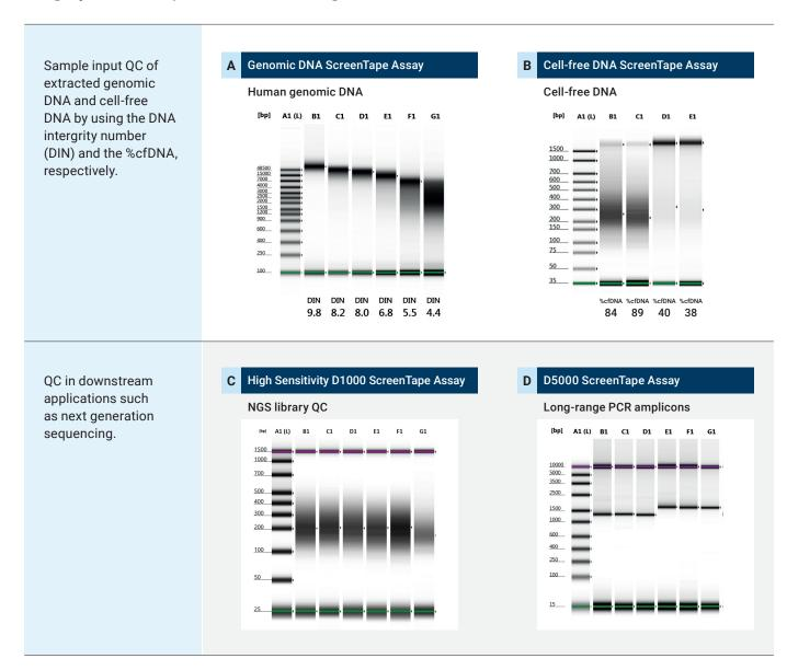
Genomic DNA smears at different degradation stages (A), cfDNA samples with different amounts of gDNA contamination (B), NGS library QC (C), and long-range PCR fragments (D).
