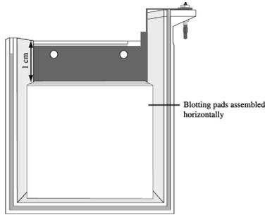
6. Hold the blot module together firmly and slide it into the guide rails on the lower buffer chamber. The blot module fits into the unit in only one way, such that the (+) sign is seen in the upper left hand corner of the blot module. The inverted gold post on the right hand side of the blot module fits into the hole next to the upright gold post on the right side of the lower buffer chamber.
