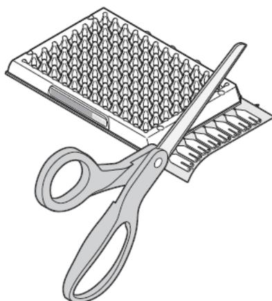
**IMPORTANT!** Completely remove the fill reservoirs from the array card so that the edge is free of residual plastic. The plastic from the fill reservoirs that extends beyond the edge of the card can prevent the array card from seating properly on the sample block and can affect amplification.
