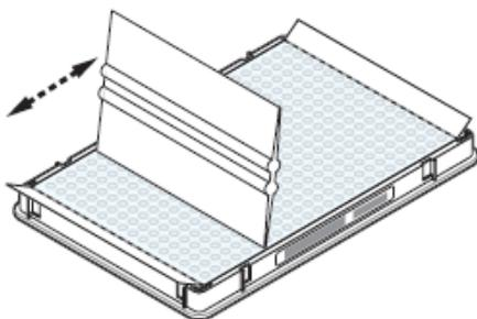
5. While using the applicator to hold the edge of the film in place, grasp one end of the end-tab and pull up and away sharply. Repeat this step for the other end-tab.
