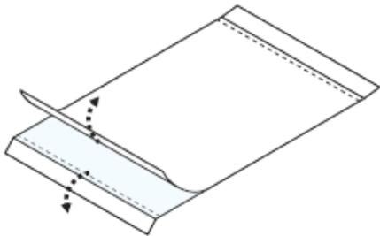
3. Holding the film by the end-tabs, lower the film onto the reaction plate (adhesive side facing the reaction plate).
