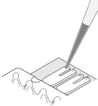
d. Dispense the fluid so that it sweeps in and around the fill reservoir toward the vent port.
