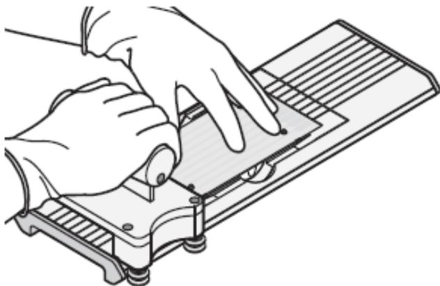
4. Seal the array card by running the carriage slowly over it. Run the carriage over the array card in one direction only. Do not apply downward force on the carriage as you move it forward over the card.
