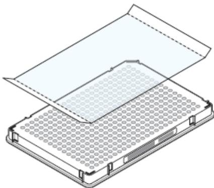
4. While applying firm pressure, move the applicator slowly across the film, horizontally and vertically, to ensure good contact between the film and the entire surface of the reaction plate.
