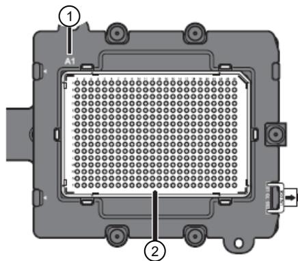
① Load 96- and 384-well plates with the A1 position at the top-left corner of the plate adapter.
