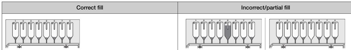
If necessary, centrifuge the array cards for an additional minute to fill any unfilled wells. Do not exceed three 1-minute runs or centrifuge the array card for longer than 1 minute at a time.
