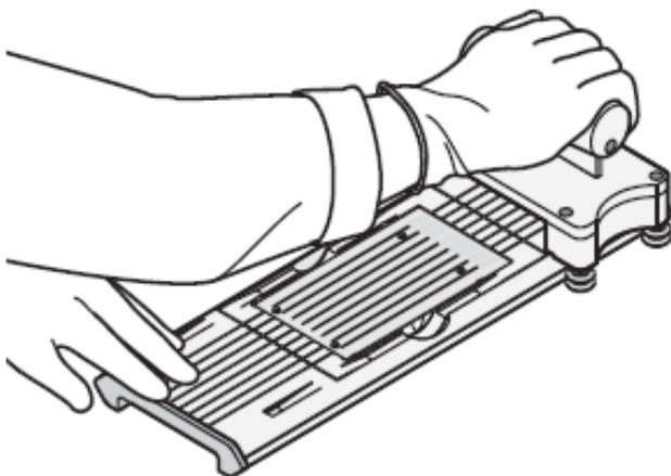
5. Remove the sealed array card from the fixture and trim the fill reservoirs from the array card assembly using scissors. Trim the foil array card so that the edge is even with the plastic carrier.
