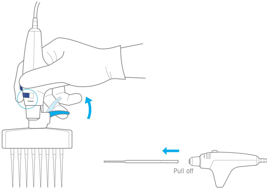
Figure 3: Ejecting Tips or removing the Pasteur pipette
