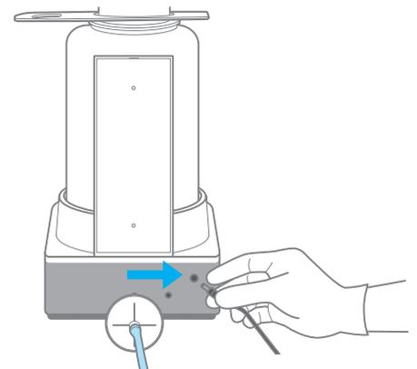
6. Load Rainin UNV 250  $\mu$ L tips or a glass (Pasteur) pipette onto appropriate adapter
