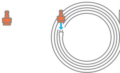
6. Attach the blue connector-plug end of the blue tube to the blue connector head by pushing it in firmly. Attach the orange connector-plug end of the clear tube to the orange connector head by pushing it in firmly.
