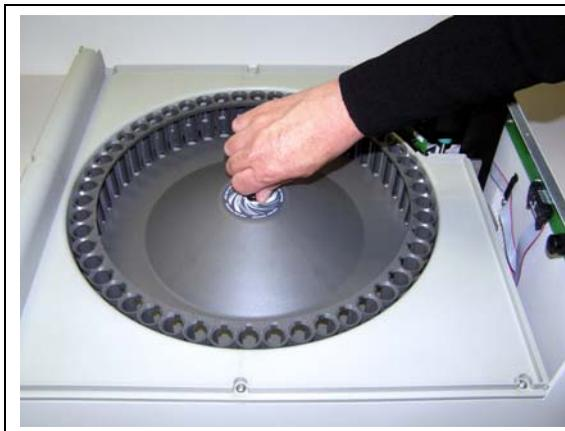
Figure 5-6. Removing the Carousel
