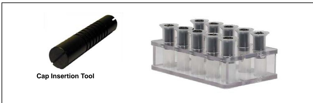
*Figure 3-3. Caps Installed (0.5 mL Vials Shown)*
