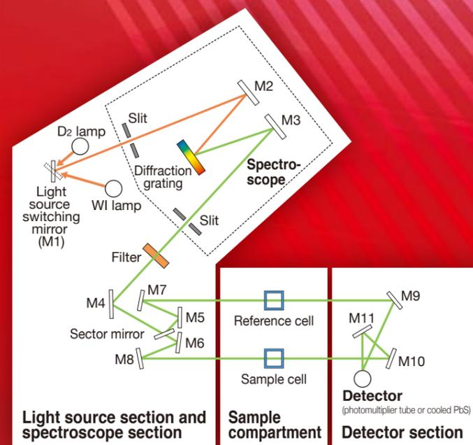
Schematic view of the UH5700 optical system
